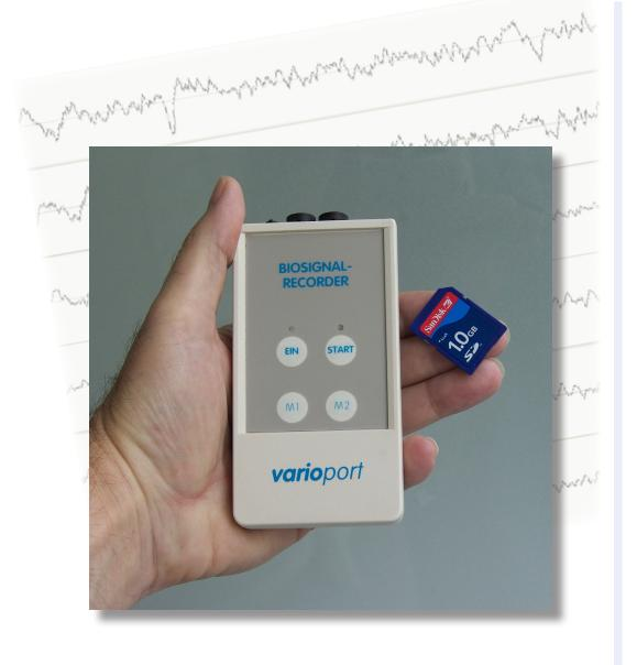
The varioport recorder system is a very small and lightweight portable measuring system. It collects physiological, movement and environmental data over a time period up to one week.
