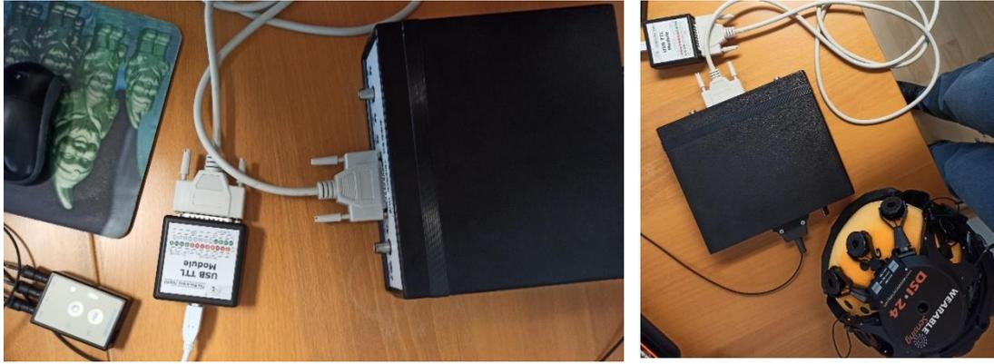
Setup Trigger Interface Box, trigger hub, varioport-e and EEG DSI-24
